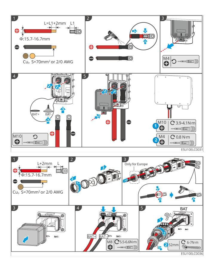
• Some models are shipped with the battery terminal screws attached to the battery
