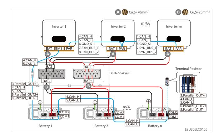
LX U5.0-30: When the battery quantity is less than or equal to 8, the connecting method for battery with the busbar BCB-32-WW-0 is used.
