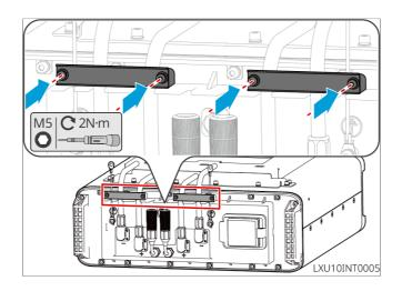
Step 2: Installing the plastic cover
