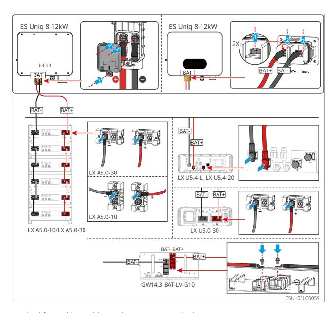
Method for making cables at the inverter terminal
