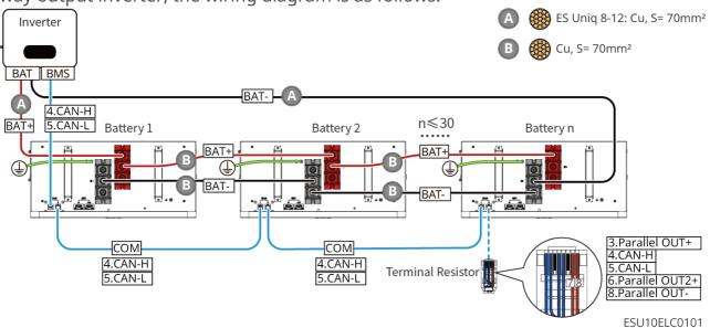
GW14.3-BAT-LV-G10: When the battery quantity is less than or equal to 15 and a busbar (BCB-32-WW-0, current <= 720A) is used to connect one way output inverter, the wiring diagram is as follows:
