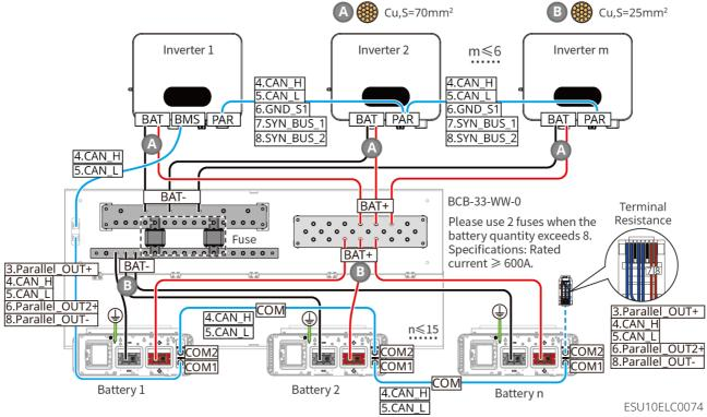
LX U5.0-30: When the battery quantity is less than or equal to 8, the connecting method with the third-party busbar is used.
