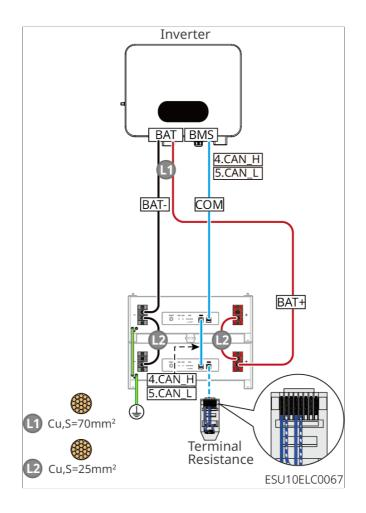
LX A5.0-10: Connecting method for battery with the busbar BCB-11-WW-0
