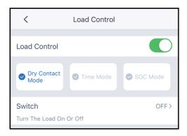
• Time Mode: set the time to enable the load, and the load will be powered automatically within the setting time period. Select standard mode or intelligent mode.
