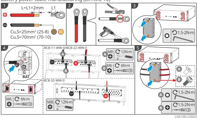
Battery power cable manufacturing (LX A5.0-30)
