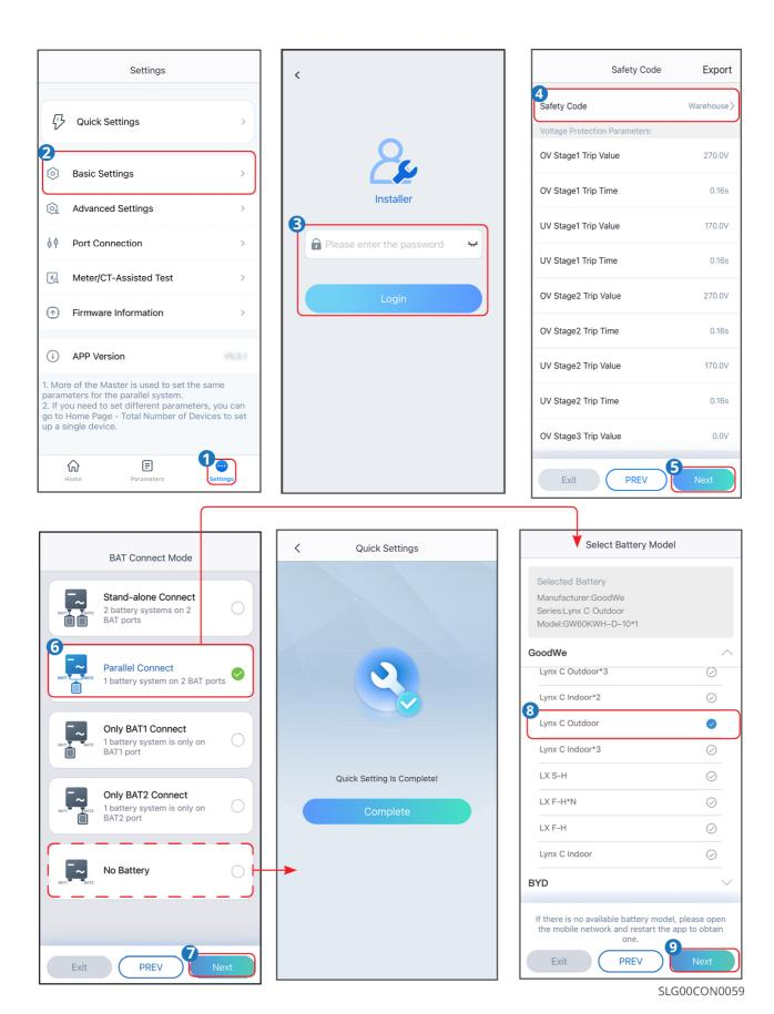
**Step 5**: Select the battery connection mode based on the actual battery connection
