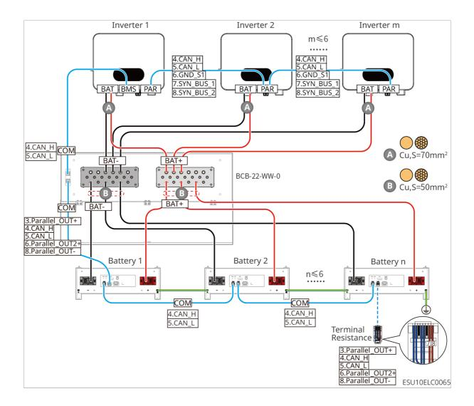
LXA5.0-30: Connecting method with the busbar BCB-32-WW-0
