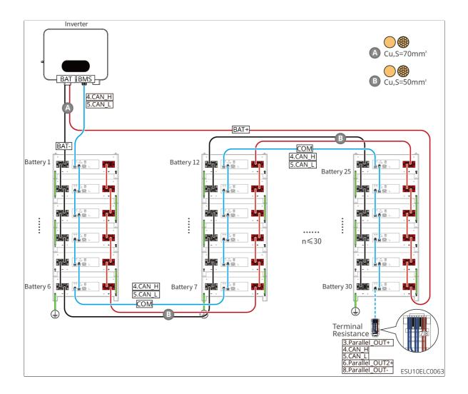
LXA5.0-30: Connecting method with the busbar BCB-22-WW-0
