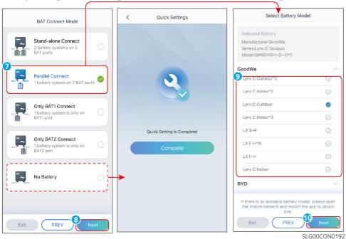
**Step 7**: Set the working mode according to actual needs. After completing the settings click **Next** to set the working mode.
