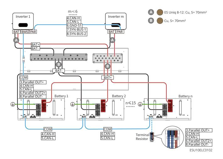
GW14.3-BAT-LV-G10: When the battery quantity is less than or equal to 30 and a third-party busbar is used to connect one way output inverter, the wiring diagram is as follows:
