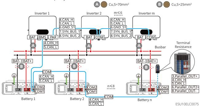
LX U5.0-30: When the battery quantity exceeds 8, the connecting method with the third-party busbar is used.
