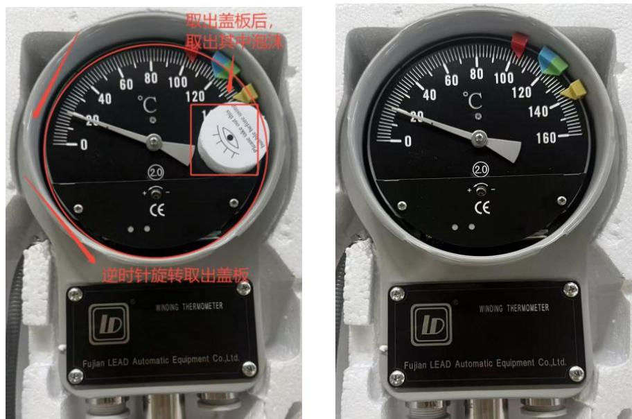
**Step 2:** Then, install the cover by rotating it clockwise. Ensure that the white needle is on the left and the red needle is on the right during installation.
