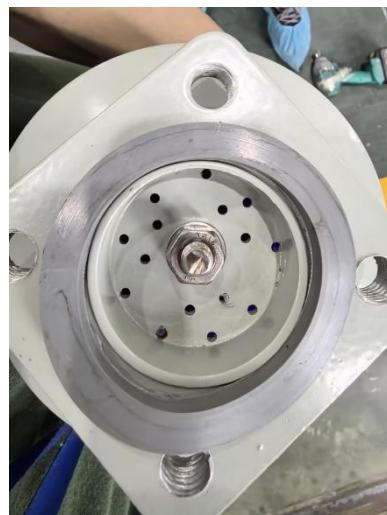
**Step 4:** Install the respirator to the breathing tube port, tighten the bolts diagonally, and install the sealing gasket as shown in the following figure.
