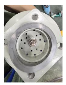
**Step 4:** Install the respirator to the breathing tube port, tighten the bolts diagonally, and install the sealing gasket as shown in the following figure.
