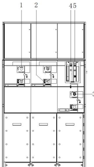
Figure 2-18 Ring main unit SAFE 12/24 CCV appearance
