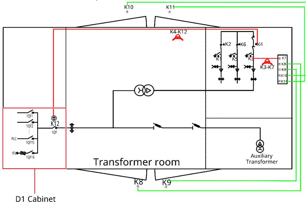
Figure 4-3 Interlocking Diagram
