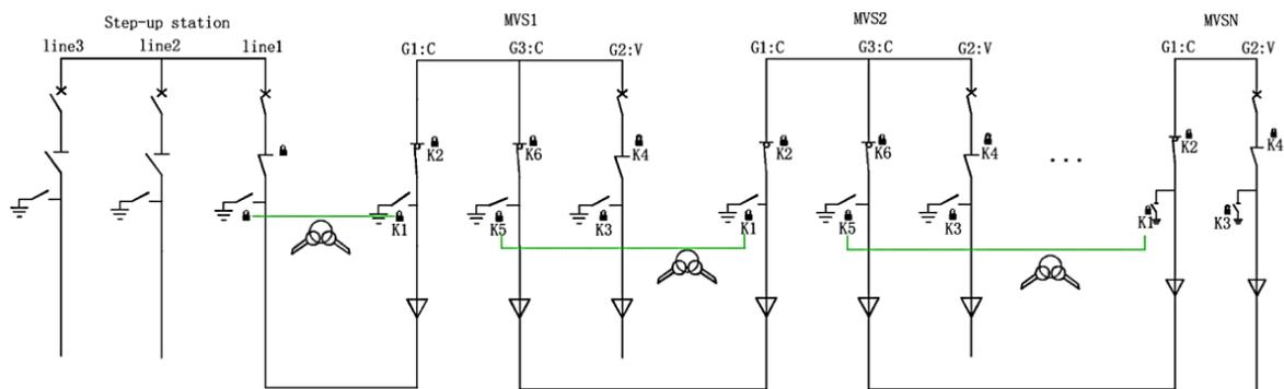
Figure 4-5 CCV type ring main unit normal interlocking
