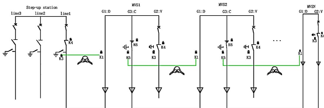
Figure 4-9 The normal interlocking of the DCV ring main unit
