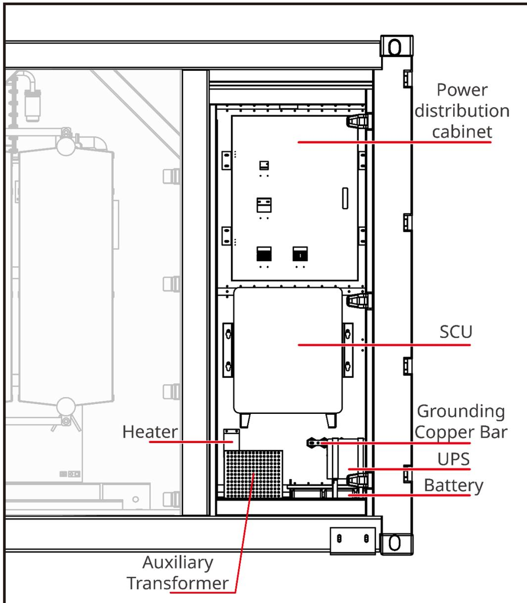
Figure 2-22 Power distribution cabinet front view layout Figure
