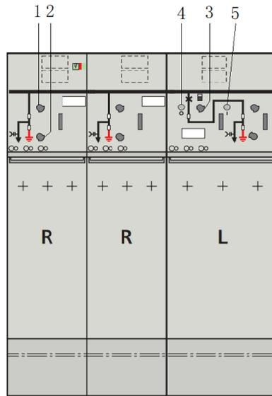
Figure 2-20 Ring main unit 24kV RRL appearance
