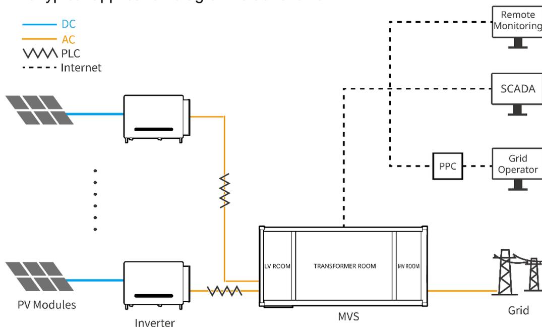
Figure 2-1 MVS Typical Application Diagram
