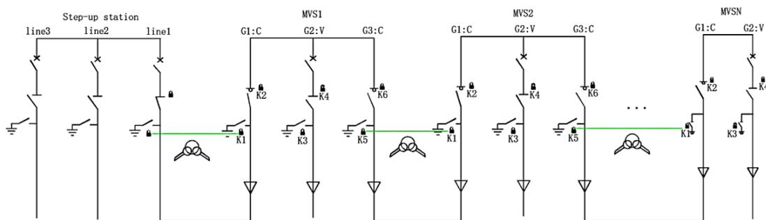
Figure 4-6 CVC type ring main unit normal interlocking
