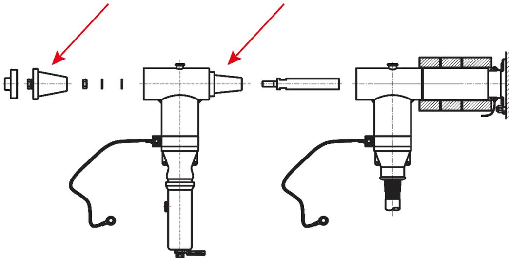
Figure 5-9 Lightning arrester and separable insulating sleeve
