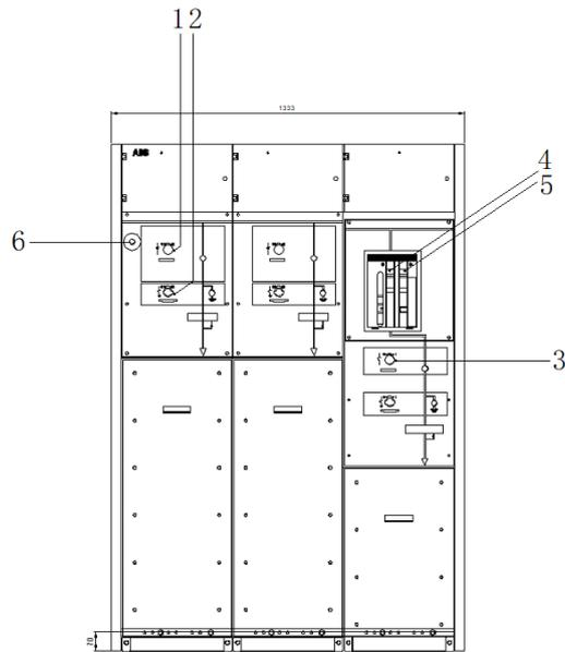
Figure 2-19 Ring main unit SAFE 40.5 CCV appearance
