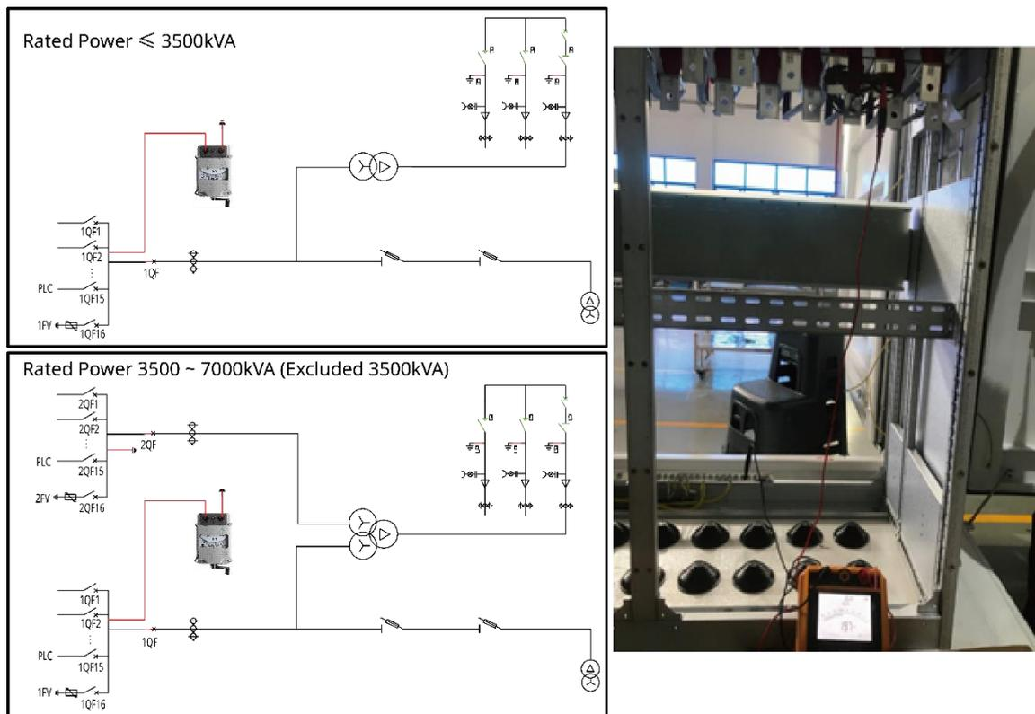
Figure 4-16 Test diagram of low-voltage cabinet D1
