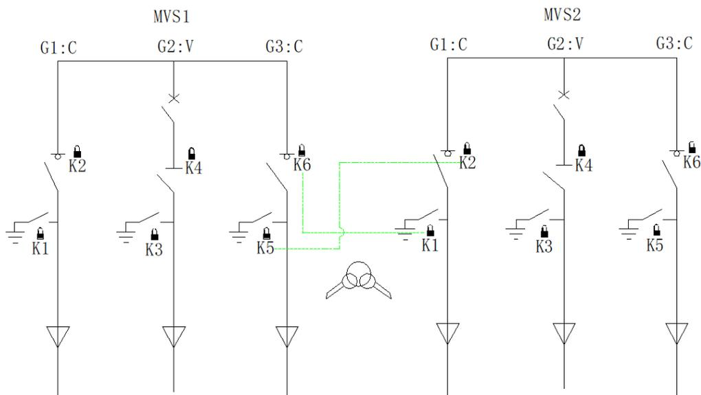
Figure 4-13 P1 Interlocking
