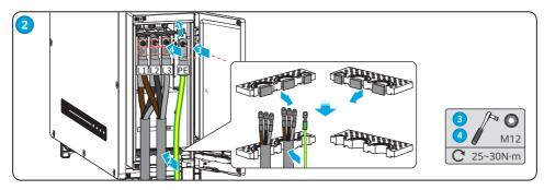
· Connecte the single-core copper cable to the terminal:
