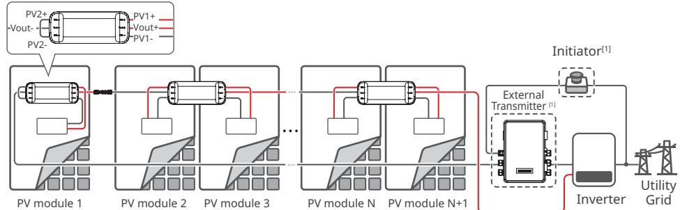
[1] Install an external transmitter and prepare an external initiator like breaker or stop button by yourself if the inverter is not integrated with an internal transmitter.
