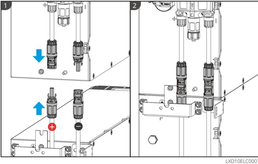
Use the package included tool and follow the steps below to remove the power connector.
